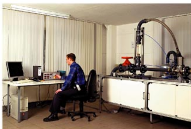
Test stand to determine and document flowrates and K_V ( C_V ) values
